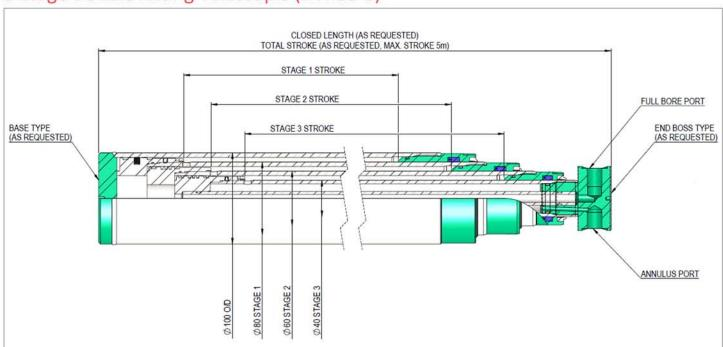
Double acting telescopic cylinders are designed to enable the retraction of the extended tube assembly under minimal load. They are not designed to pull heavy loads and are speed restricted due to the internal back pressures generated inside.
